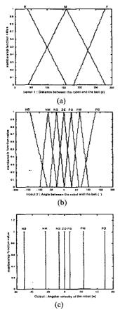
Fig. 3. Fuzzy sets for the tracking control system (a) Input: Membership function for d (b) Input: Membership function for (c) Output: membership functions for  $\omega$
