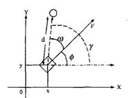
Fig. 2. The relationship between the ball and the robot
