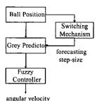
Fig. 1. Block diagram of the switching grey prediction fuzzy tracking system
